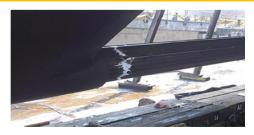
Minimization of launch induced deflection by installation of technical shaft to simulate the solid reference axis (Pre-alignment condition) for facilitating completion of structural shafting job on slipway before launching.
